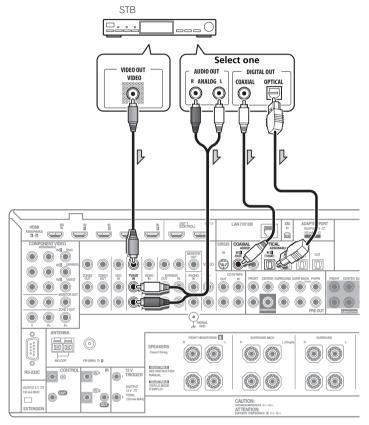
• If your set-top box is equipped with an HDMI output terminal, we recommend connecting it to the receiver's **HDMI IN** terminal. When doing so, also connect the receiver and TV by HDMI (see *Connecting using HDMI* on page 24).
